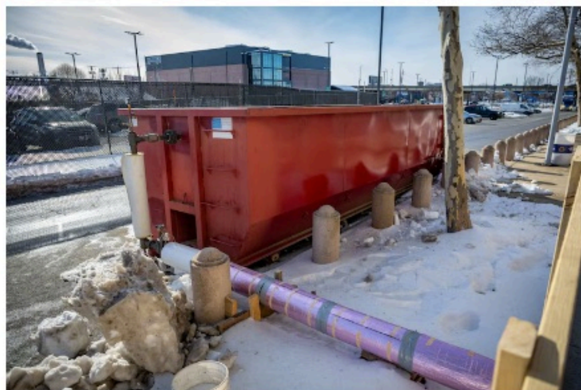
A snow melter tied into a steam line is seen outside M&T Bank Stadium. (Jerry Jackson/The Banner)
